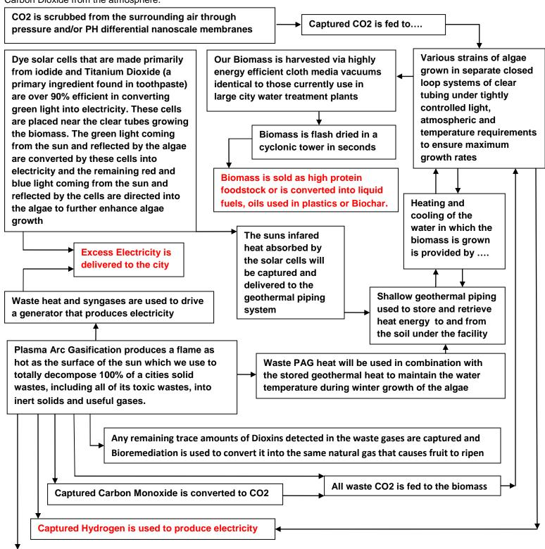
Vitrified inert solids are crushed and sold as additives to bricks, cement and asphalt
